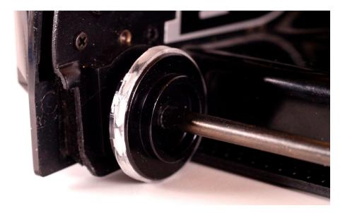
**Step 4:** Reassemble the roller, retaining plate, and two screws. If the band ever slips off the wheel, you'll have to take these parts off again and re-position it.
