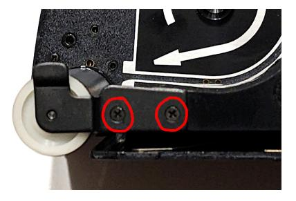
**Step 2:** Remove the metal plate held by the screws and the roller.
